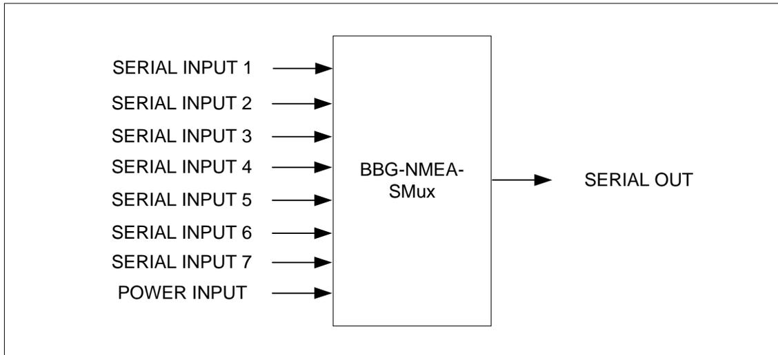
The BBG-NMEA-SMux operates on +24 VDC input power and performs serial combining of up to seven (7) NMEA-0183 serial inputs into one NMEA-0183 serial output. Input and output baud rates are switch selectable and status LEDs show input activity and system status
